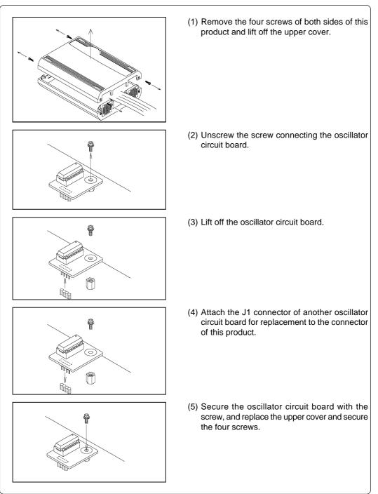
Figure 3.6 Replacing the oscillator circuit boards
